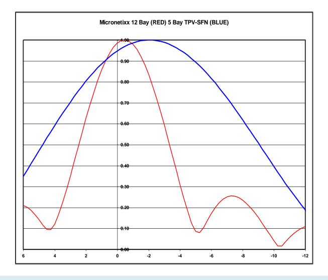
The graph above shows the elevation plots of two antennas, the 12-Bay analog antenna in service, (RED plot), and the new 5-Bay antenna we are studying (BLUE plot). With the 5-Bay antenna we were able to add more beam tilt, (3.50 degrees), and still keep the peak field at the horizon at about 94%. In the good old analog days the station wanted to get out as far as possible. Having as much signal as possible was the way to go.
